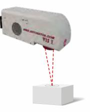
**DOUBLE LASER POINTER SYSTEM** for visually identifying the correct focal distance.
